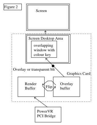
The above diagram shows how an application can use SGL's Address mode to render into an offscreen overlay buffer. The application must create and manage the buffers.
