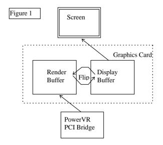
Two buffers are used, one is the on-screen display buffer and the other is the off-screen back-buffer. PowerVR renders to the back buffer while the front buffer is being displayed. When PowerVR has finished rendering the buffers are switched and the rendered image becomes visible. A third buffer may be used, if there is enough off-screen memory, to avoid having to wait for Vsync during the buffer switching process.
